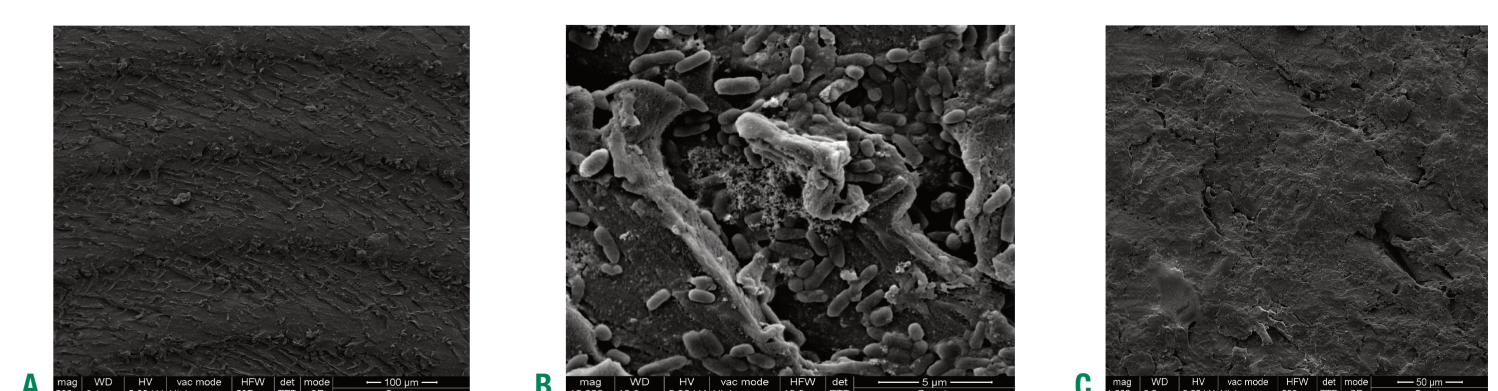
Figure 4. Electron micrograph images P. aeruginosa that had been encouraged to form a biofilm on CDC coupons. Coupons were negative (A) untreated (B) and treated with the novel treatment method (C).
