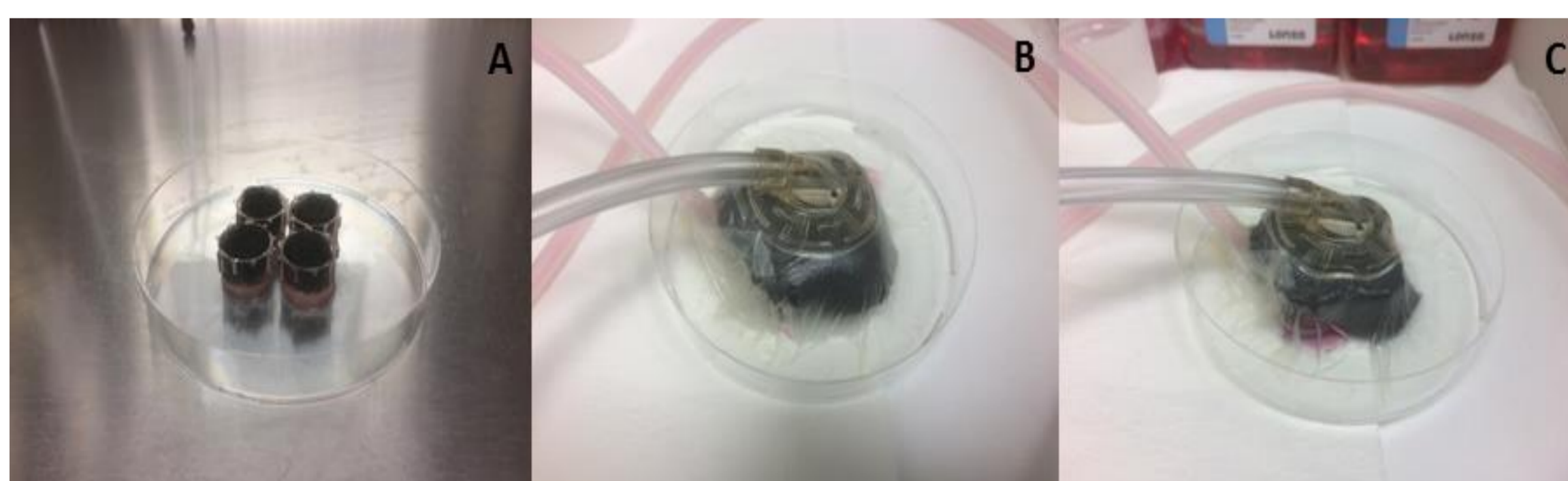
Figure 1: For NPWT the hDF-3d-cultures were positioned in a Petri dish (A), connected to medium supply and sealed airtight with V.A.C.® Drape (B) before the set-up was linked to the vacuum pump KCI* (C).
